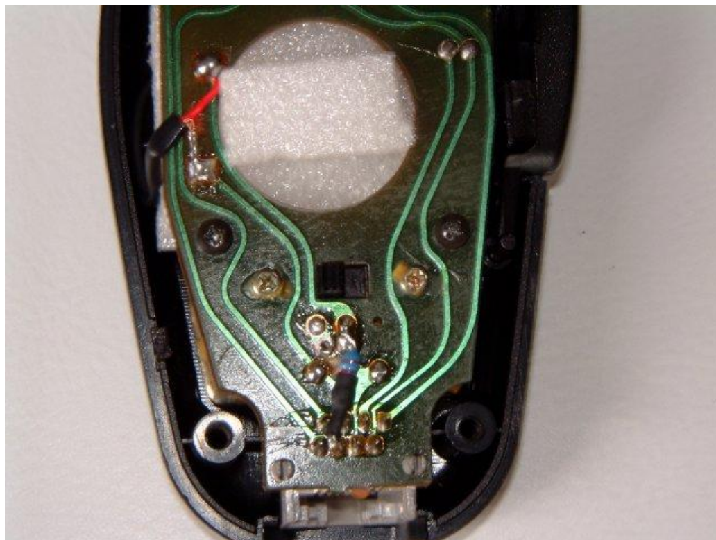
Resistor for the DC power supply of the capsule on the upper side of the PCB.
